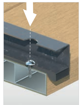
Screw in in the extra thickness of the profile
