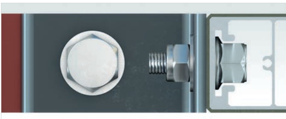
Example for fastening assembly brackets (not supplied) using braked nuts.
