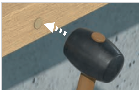
Press caps with a rubber mallet
