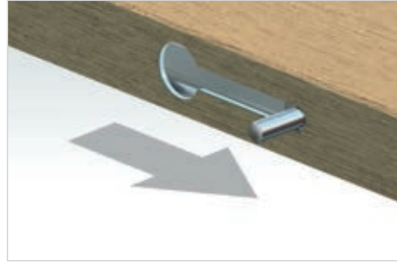
Setting up the first flange bolt.
